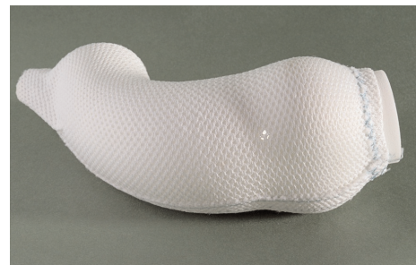
MAIN IMAGE: EARS SLS former with textile implant
