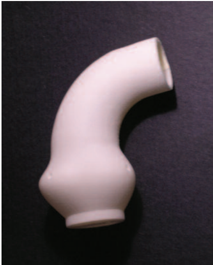
Figure 1b: The model is used to sculpt by rapid prototyping a replica of the individual's aorta.
